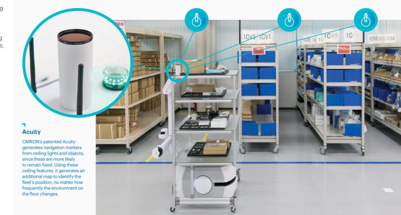
Our safe and intelligent navigation leads the industry in speed and accuracy. Using multiple systems, our robots learn to become even more efficient after they're installed. Every robot in our fleet acts as a sensor to map out the most challenging environments and optimize its performance, from navigating tight aisles to planning the most efficient routes.
